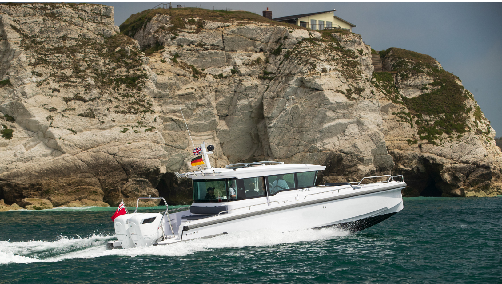
Axopar 37 powered with twin CXO300 diesel outboards
