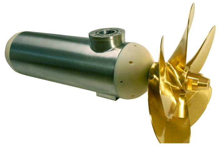
Fischer Panda UK has extended its drive system portfolio with the introduction of a new 100 kW electric motor
