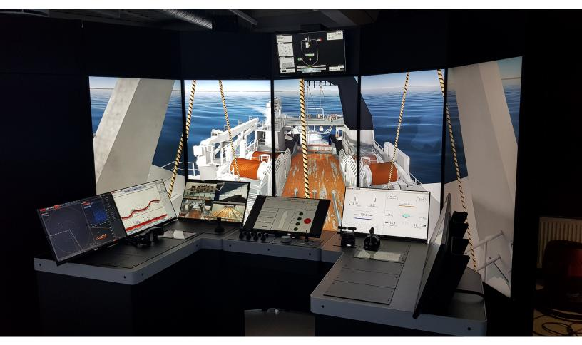
The new K-Sim Fishery simulator includes instruments and aft deck view enabling training to avoid risk elements associated with aft deck operations onboard fishing vessels
