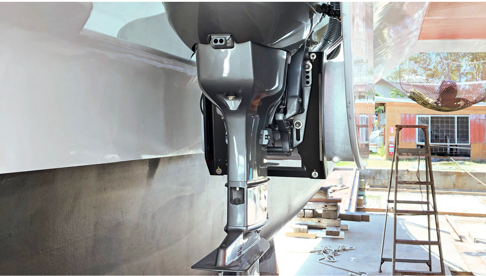
One of the YANMAR Neander Dtorque diesel outboards mounted mid-hull on sailing catamaran X-IT
