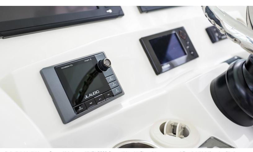
JL Audio's MediaMaster Source Unit is now NMEA 2000 Compatible with Simrad, Lowrance and Garmin's Multifunction Displays
