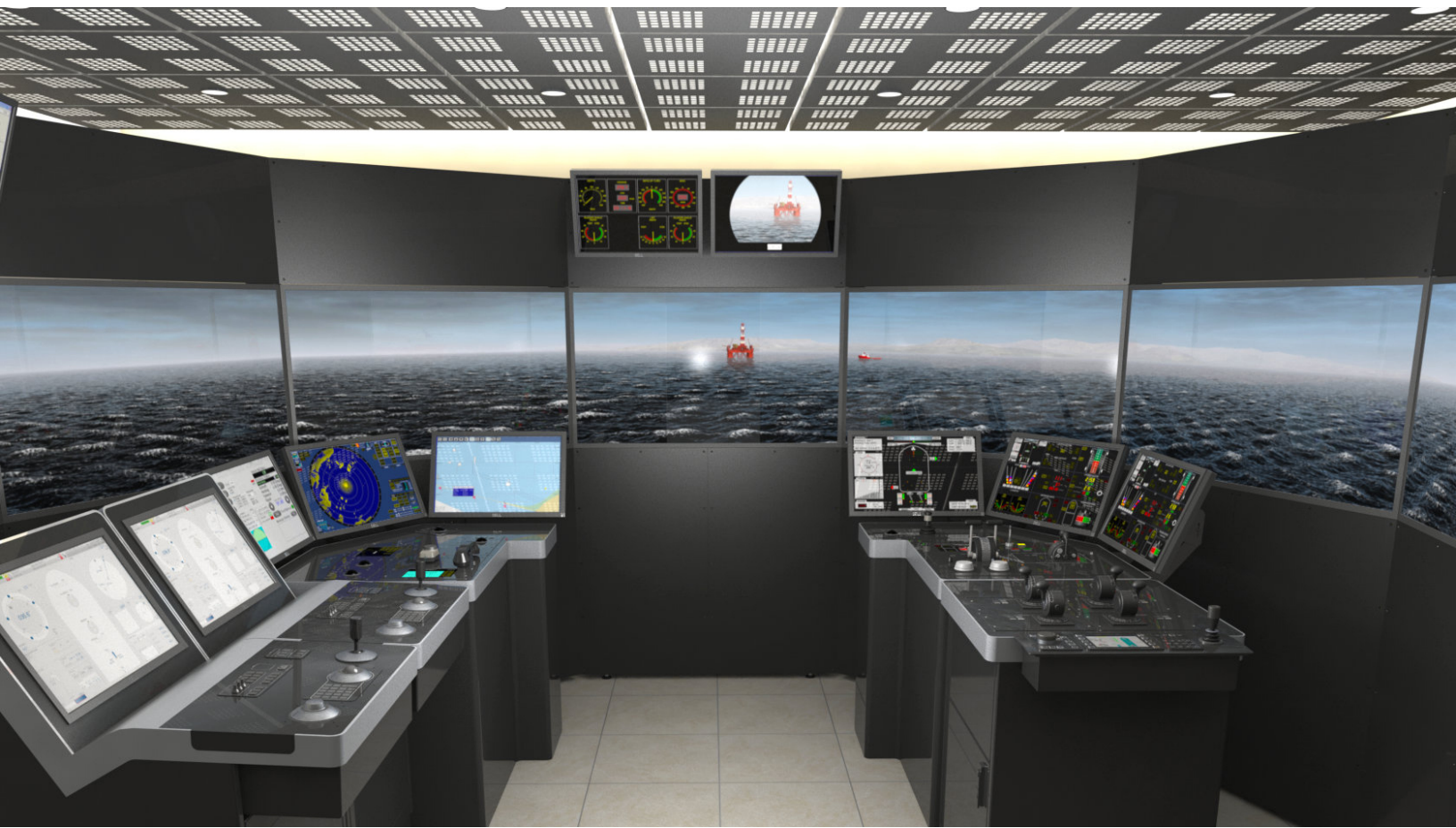
An aft bridge simulator, similar to the one which is a part of the KONGSBERG delivery to Maritime Campus North
