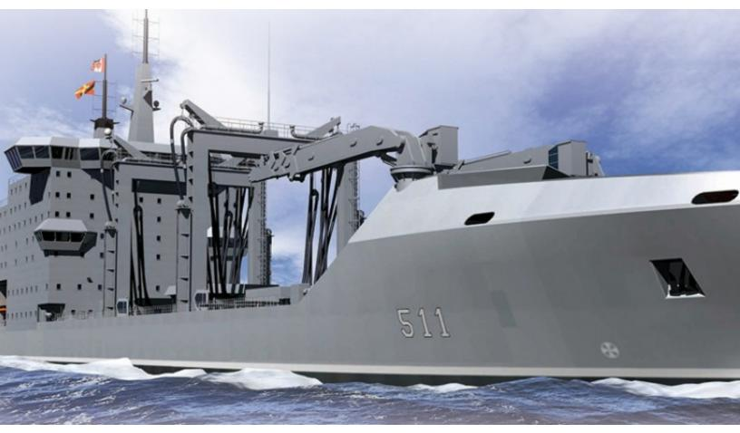
'Project Resolve' is based on a conversion of the commercial container ship, 'MS Asterix'
