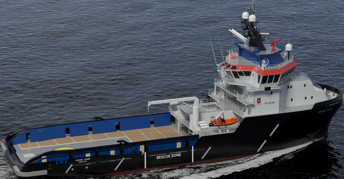
Kongsberg Maritime's 71.6-metre UT 722 tugboat design has bollard pull of 200 tonnes and can operate as a long-range towing vessel in the Suez Canal and the Mediterranean Sea
