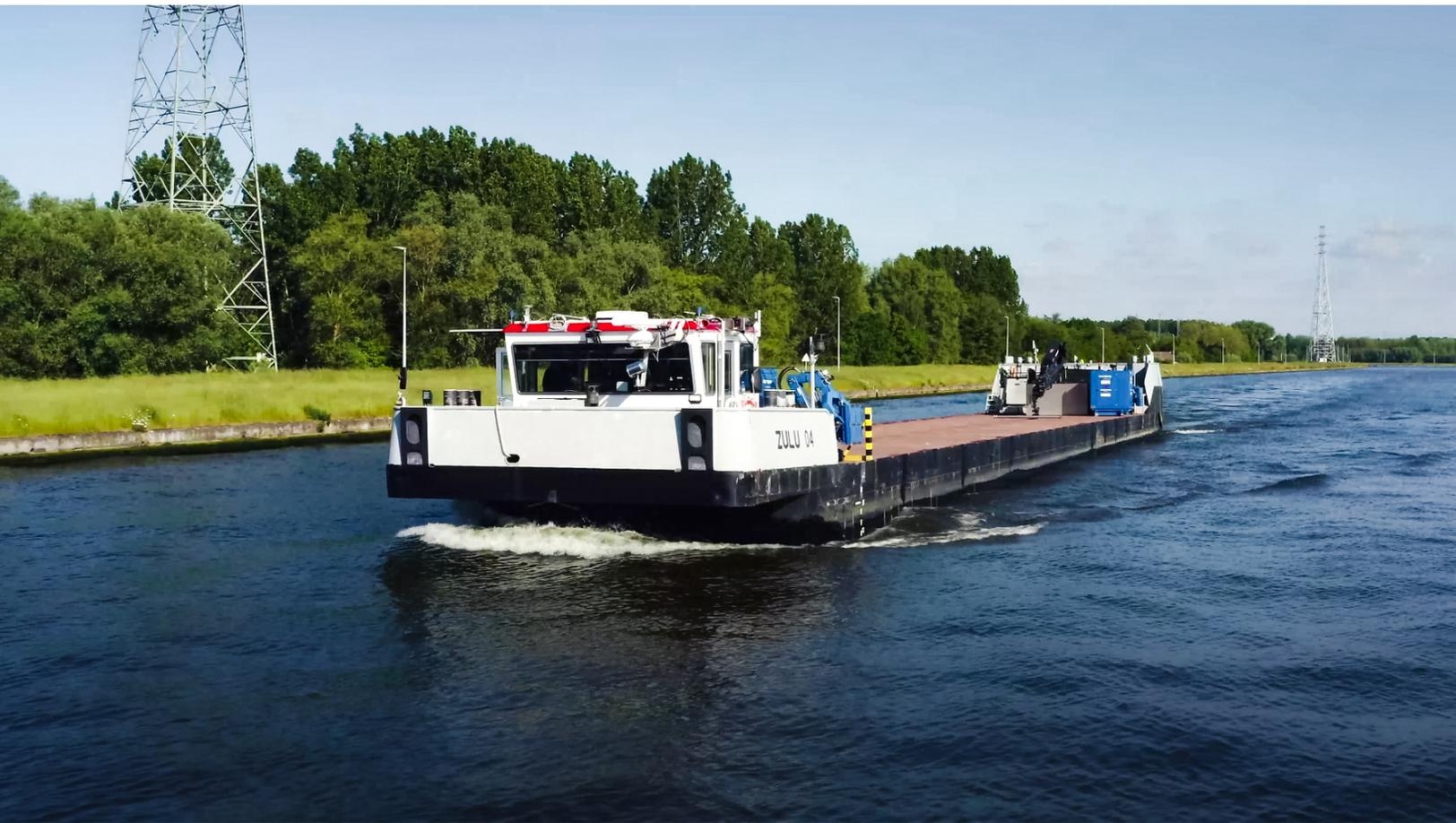
The Zulu 4 canal vessel completed a 16.5-kilometre circuit using autonomous and remote operations technology
