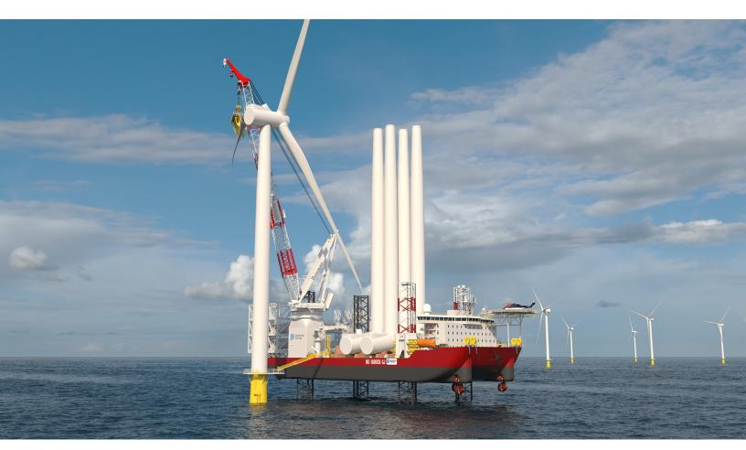
Dominion Energy's new Wind Turbine Installation Vessel, due for delivery by the end of 2023, will be built by Keppel AmFELS and fitted with Kongsberg Maritime's field-proven integrated solution for WTIV operation
