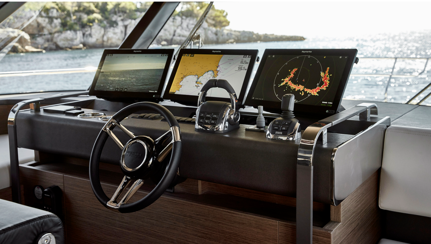
Three Axiom XL 16-inch MFDs on the PRESTIGE X70 - Photo Credit: Jean-Francois Romero
