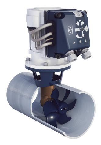
VETUS New BOWA0401 for 140mm tunnels, suitable for vessels 9m and under
