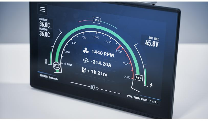
VETUS battery monitoring shunt and multifunction display enables crucial visibility of the remaining battery charge and runtime
