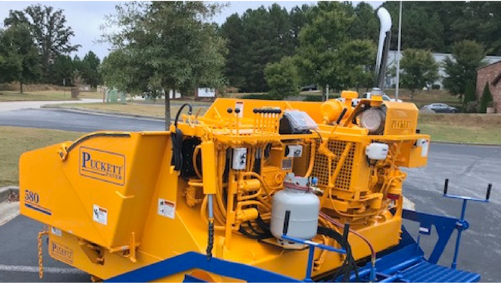
The Puckett 580 asphalt paver with customized 3TNV88C-DYEM YANMAR Tier 4F engine from YANMAR Mastry Engine Center
